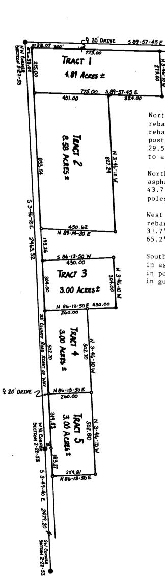
North Quarter Corner of Sec. 2-22-53, found a 5/8" rebar 3' below surface of county road, set 5/8"x 24" rebar over it, 26.3' S to a spike in top of a corner post, 33.2' SW to a spike in top of a gate post, 29.5' N to a spike in a corner post and 37.4' NW to a spike in a gate post.
