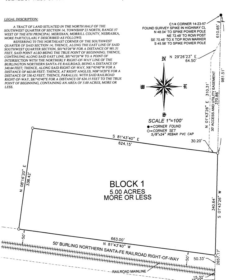
S1/4 CORNER 14-23-57 FOUND RR SPIKE IN COUNTY ROAD NW 48.29' TO SPIKE FENCE POST NE 50.83' TO SPIKE FENCE POST ESE 80.55' TO SPIKE POWER POLE SW 49.96' TO SPIKE FENCE CORNER
