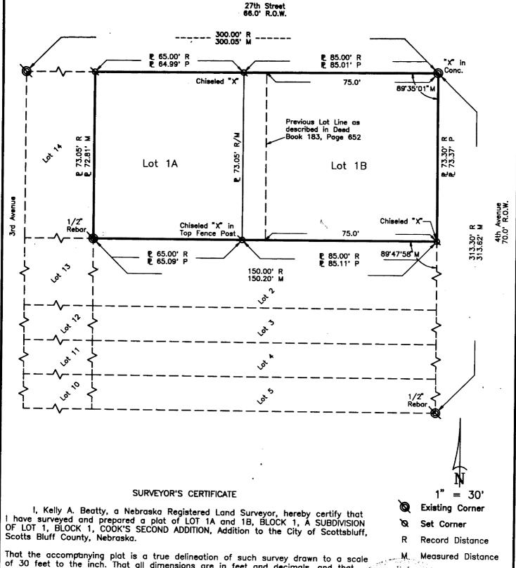
That the accompanying plat is a true delineation of such survey drawn to a scale of 30 feet to the inch. That all dimensions are in feet and decimals, and that each lot and block has its own number. That the boundary of the plat is shown with a heavy solid line with dashed lines being for orientation purposes only. That all corners found or set are marked as shown.
