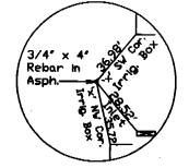
North Quarter Corner Sec. 25, T22N-R55W Exist. 5/8" Rebar in Asphalt
