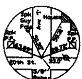
WEST QUARTER CORNER Section 23, T22N-R55W Found \frac{1}{2} " Rebar
