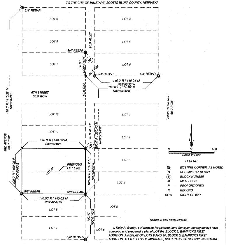
5TH STREET 60.0' ROW That the accompanying plat is a true delineation of said survey drawn to a scale of 50 feet to the inch. That all dimensions are in feet and decimals. That each lot and block has its own number. That the boundary of the plat is shown with a heavy solid line with dashed lines being for orientation purposes only. That all corners found or set are marked as shown.
