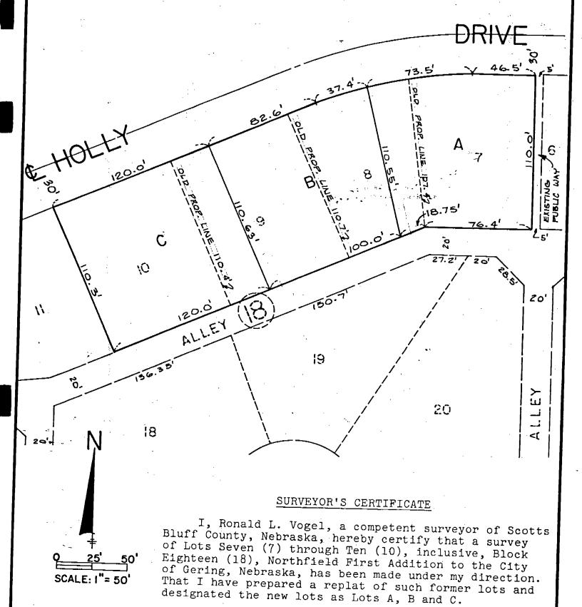
That the accompanying plat is a correct delineation of such survey, drawn to a scale of 50 feet to the inch, with all dimensions shown thereon in feet and decimals. That each new lot bears its own letter and that iron rods are driven well into the ground at all corners of the lots. That the boundary of the subdivision is shown on the plat with a heavy solid line and that adjoining lots are shown dashed for orientation purposes.
