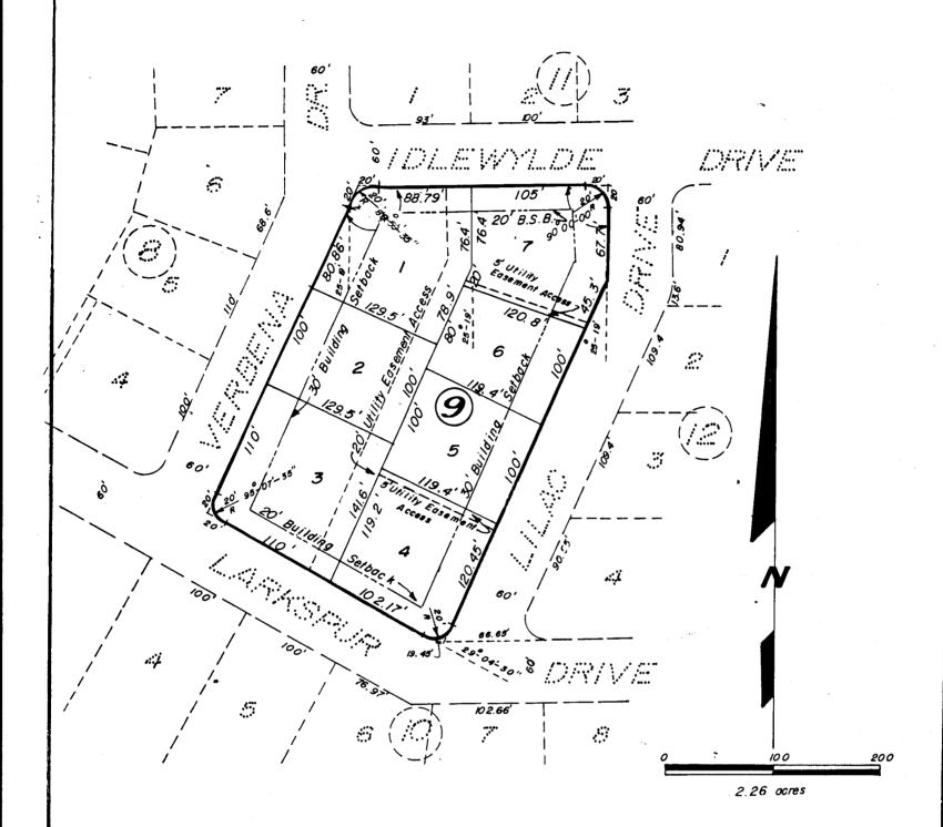
NOTE: All lot Corners were set with 3/4"x 18" rebar and all Block Corners were set with 3/4"x 36" rebar.
